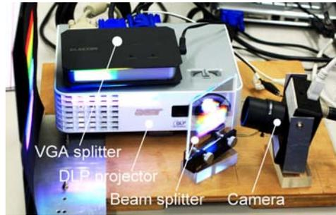
**Figure 1.** System Configuration of the Proposed Spatial-projection Display.
